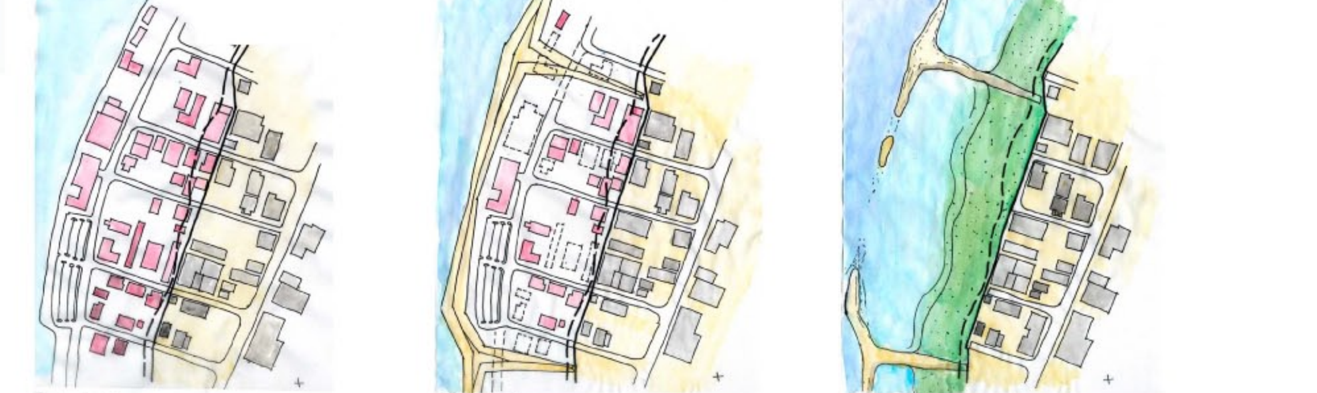
2009 In this sketch the conditions in 2009 are shown. A sea wall and fill has created flat urban zones. There are parking lots, industrial facilities and residential properties in areas that are certain to be flooded. 2035 Non-permanent levee have been constructed and the properties behind the levees are being relocated or deconstructed. 2050 Present Levees were breached and wetlands are established in once urban areas. Levees are in the process of erosion into sandbars
